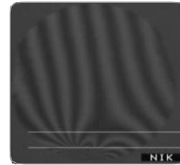
1,000 \mu\text{m} diameter fiber Interference microscope image 1 stripe = 0.01°
